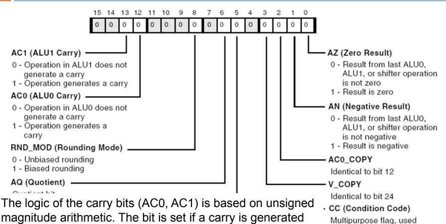
primarily to hold resolution of arithmetic comparisons. Also The carry bits (AC0, AC1) are most useful for the lower used by some shifter instructions to hold rotating bits. word portions of a multiword operation.
