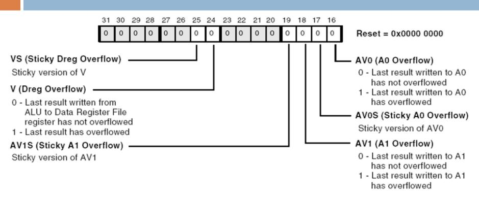
The logic of the overflow bits (V, VS, AV0, AV0S, AV1, AV1S) is based on two's-complement arithmetic. A bit or set of bits is set if the Most Significant Bit (MSB) changes in a manner not predicted by the signs of the operands and the nature of the operation.
