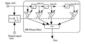
The Wiener filter error signal, e(m) is defined as the difference between the desired signal x(m) and the filter output signal x^ (m) :
