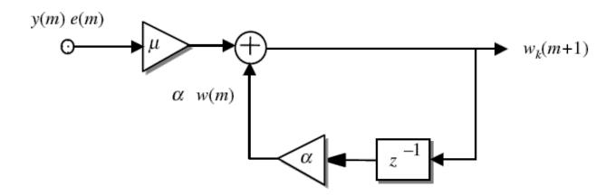
Note that the feedback equation for the time update of the filter coefficients is essentially a recursive (infinite impulse response) system with input μ[y(m)e(m)] and its poles at α.
