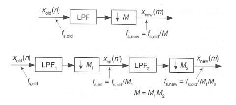
What should be the values of  $D_1$  and  $D_2$  to minimize the number of taps in lowpass filters LPF<sub>1</sub> and LPF<sub>2</sub>?
