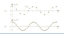
Interpolation is the two-step processes of an operation know as upsampling followed by low-pass filtering.
